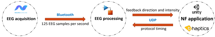
Figure 2: Block diagram of the wearable brain-computer interface. The information exchanged between blocks (black) and the exploited communication protocols (blue) are highlighted. EEG: electroencephalography, UDP: User Datagram Protocol, NF: neurofeedback.
