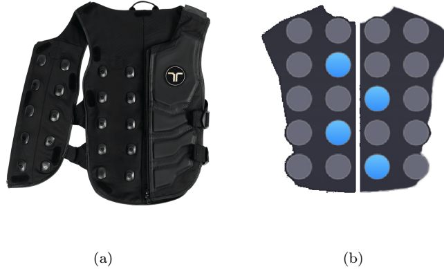
Figure 4: Wearable and portable haptic suit with a double vibration motors matrix: (a) suit, (b) front view of matrix with motors.
