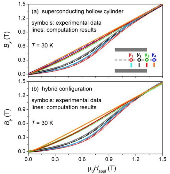
Fig. 3. Comparison between the  $B_y$  values measured in the transverse-field configuration by the Hall probes at  $T = 30$  K and the corresponding curves computed by numerical simulations for the SC hollow cylinder alone (a) and for the hybrid shield (b). No experimental data are shown for the hybrid configuration at position  $y_4$  due to a failure of the related Hall probe.
