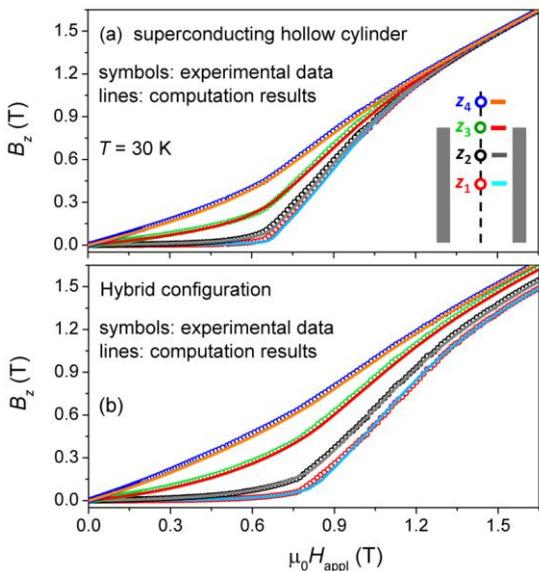
Fig. 2. Comparison between  $B_z$  values measured in the axial-field configuration by the Hall probes at  $T = 30$  K and the corresponding curves computed by numerical simulations for the SC hollow cylinder alone (a) and for the hybrid shield (b).
