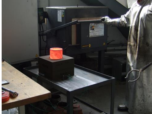
Figure 13: F-TPS finished sample during thermal test, [2].
