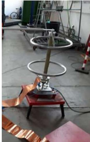
Fig. 1. SAGI 304 resistive divider up to 200 kV.
