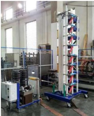
Fig. 2. LATFC's Haefely Impulse generator.
