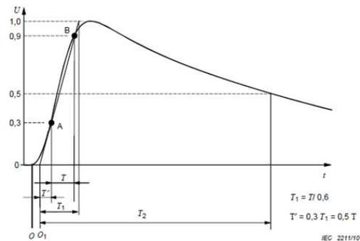
Fig. 3. Lightning impulse time parameters, from IEC 60060-1
