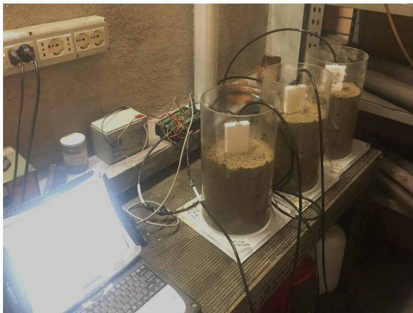
Figure 1. Experimental setup. The three columns are the three mesocosms. A white TDR probe is inserted in each of them and connected to the black datalogger behind.
