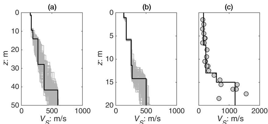
**Fig. 1.** Results of the MASW tests carried out along the crest of the Arignano (a) and Briaglia (b) dams (the thick lines are the minimum misfit profiles); (c) results of the DH test performed on the Briaglia dam.
