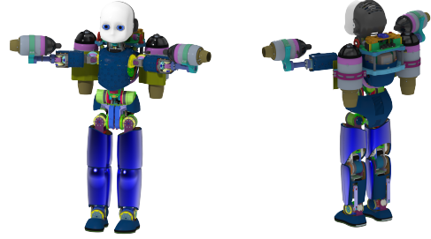
Fig. 1. iRonCub: the jet-powered humanoid robot. The jets are attached to the arms and the chest and exert 160 N and 220 N respectively.
