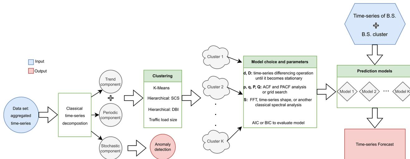
FIGURE 3. General procedure to obtain SARIMA(p, d, q)(P, D, Q)<sub>S</sub> models for network traffic prediction.
