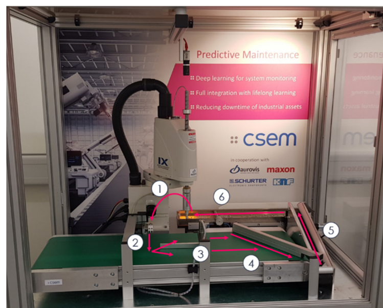
Figure 1. Equipment: 4-axis SCARA-robot picking up electrical fuses with a vacuum gripper, from a feeder to a fuse-test-bench for a large-scale quality-control. Arrows represent the main phases involved in the quality-control process: (1) picking up, (2) thermal camera control, (3) sorting, (4), (5) transport and (6) storage.
