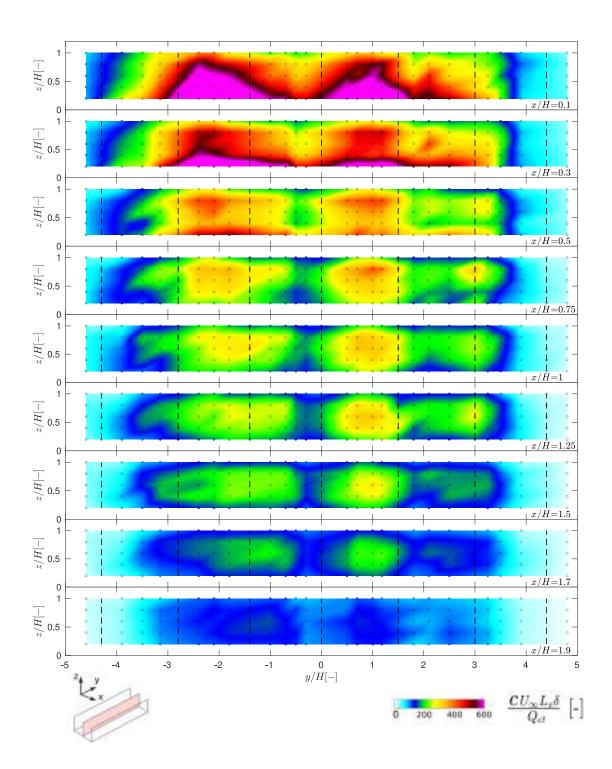
Figure S4: Configuration *Half.* Mean concentration of the passive scalar on vertical sections at different x positions. The position of trees is represented by dashed lines. Measurement points are reported as circles coloured according to the measured value.
