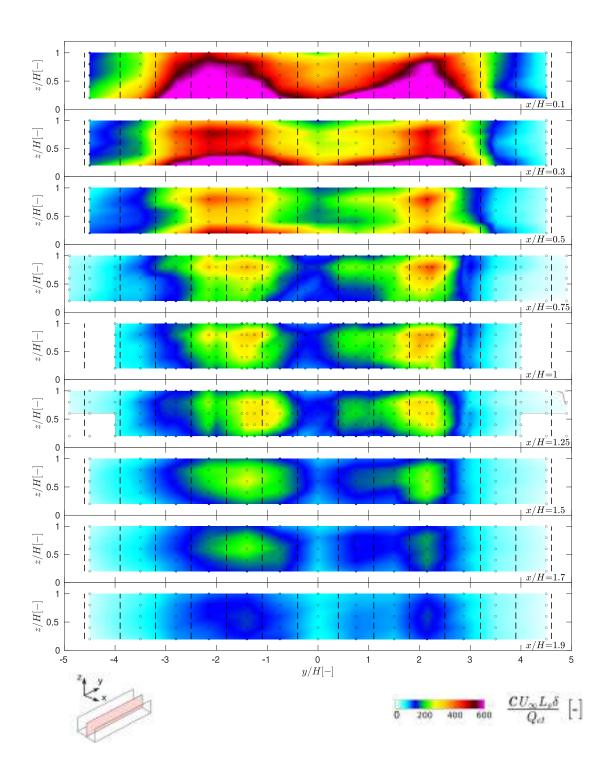
Figure S5: Configuration *Full.* Mean concentration of the passive scalar on vertical sections at different x positions. The position of trees<sup>7</sup> is represented by dashed lines. Measurement points are reported as circles coloured according to the measured value.
