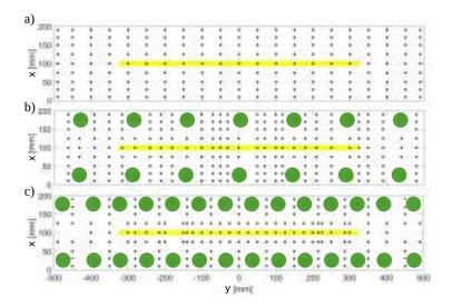
Figure S2: Sketch of the street canyon with the three different configurations of tree density: a) Zero, b) Half, and c) Full. The measurement grid is also shown for one of the five horizontal planes at fixed z.
