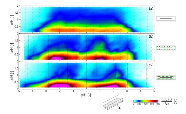
Figure S6: Mean concentration of the passive scalar on the horizontal section at z/H=0.2. Zero (a and d), Half (b and e) and Full (c and f) configurations are shown. The position of trees is represented by dashed lines. Measurement points are reported as circles colored according to the measured value.
