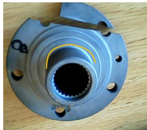
Fig.3 - Real image of the wheel's hub after nitriding and sample cutting for metallographic analysis. The yellow line shows the notch area subjected to induction hardening and shot peening.
