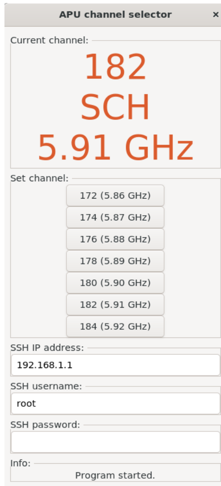
Figure 3.4: DSRC platform channel selector GUI tool. This tool can be used to easily select any DSRC channel on an APU board, connected to the PC running the GUI via ssh.
