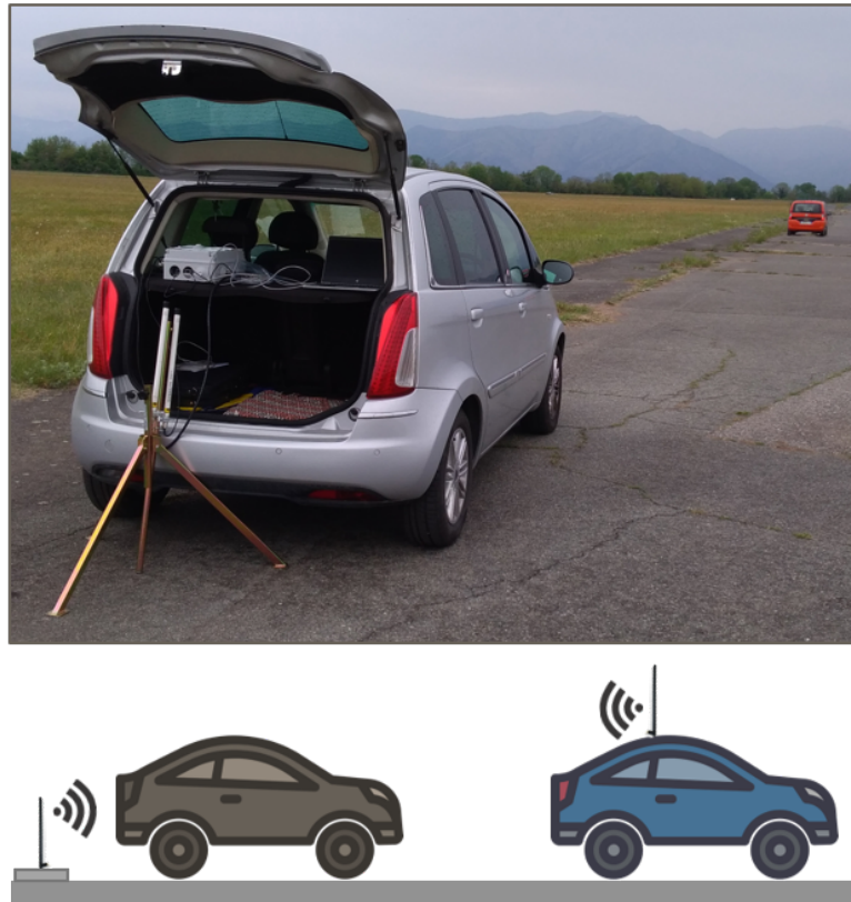
Figure 4.19: Test setup for measurements under NLOS conditions.
