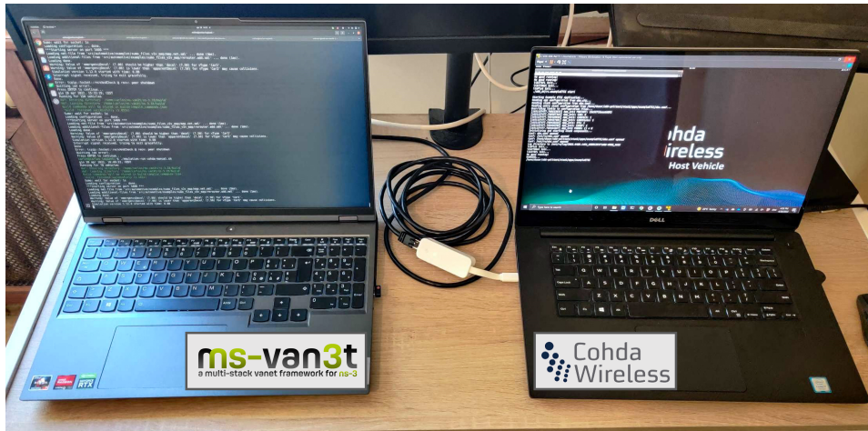
Figure 4.7: Laboratory setup for the interoperability tests between ms-van3t and a commercial, automotive-grade, ETSI ITS-G5 stack. These tests allowed us to validate the emulation feature available in ms-van3t.
