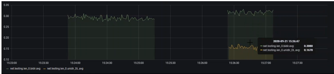
Figure 3.6: Example of a simple Grafana dashboard, showing average latency data from a LaTe test over the loopback interface. Both bidirectional and unidirectional latency, coming from two parallel LaTe client-server sessions, are displayed.
