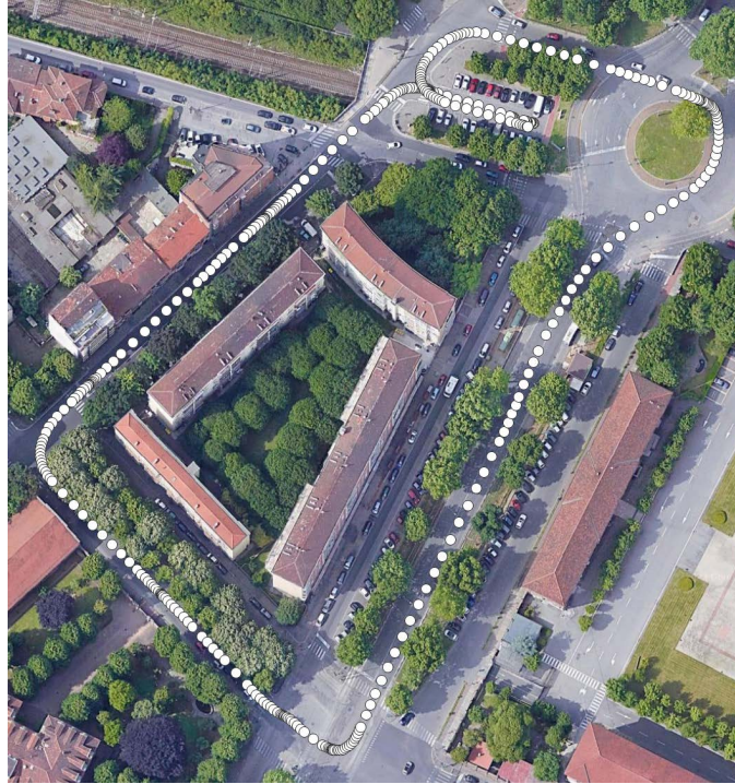
Figure 3.17: Trace of a vehicle equipped with the open OBU prototype during a test in Turin, Italy. Each white dot correspond to the position where a CAM message was transmitted.
