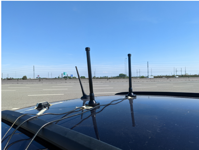
Figure 3.19: Antenna setup on the roof of our vehicle (Fiat Panda) for the interoperability and motorway tests with our OBU prototype.
