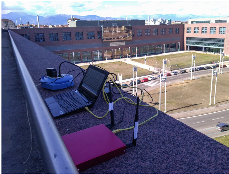
Figure 3.8: Picture showing one APU1D board with the IEEE 802.11p platform, and one laptop interfaced with the board through Gigabit Ethernet, in the place where the outdoor tests have been performed.
