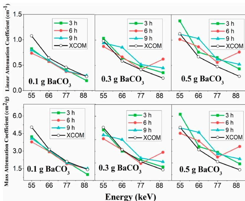
**Figure 20.** The experimental values of linear attenuation coefficient ( $\mu$ ) and mass attenuation coefficient ( $\mu_m$ ) for different delignification times and  $\text{BaCO}_3$  content (filled symbol indicated by 3, 6, and 9 h). For comparison, the theoretical calculation (XCOM database) from the National Institute of Science and Technology (India) (open symbol) is included. Reprinted with permission from [40], copyright 2022, Elsevier.
