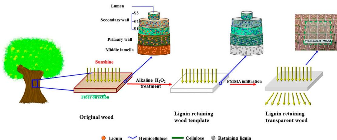
**Figure 6.** Schematic of process of obtaining transparent wood by lignin modification followed by PMMA infiltration. Reprinted with permission from [31], copyright 2017, John Wiley & Sons.
