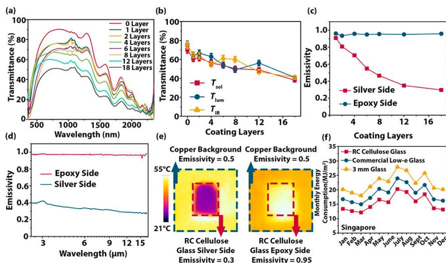
**Figure 28.** (a) UV-vis-NIR spectra of the radiative cooling transparent bamboo with various numbers of silver nanowire layers; (b) integrated  $T_{sol}$  (solar transmittance),  $T_{lum}$  (luminous transmittance), and  $T_{IR}$  (infrared transmittance) values of the radiative cooling transparent bamboo as a function of the number of silver nanowire layers; (c) emissivity of the radiative cooling transparent
