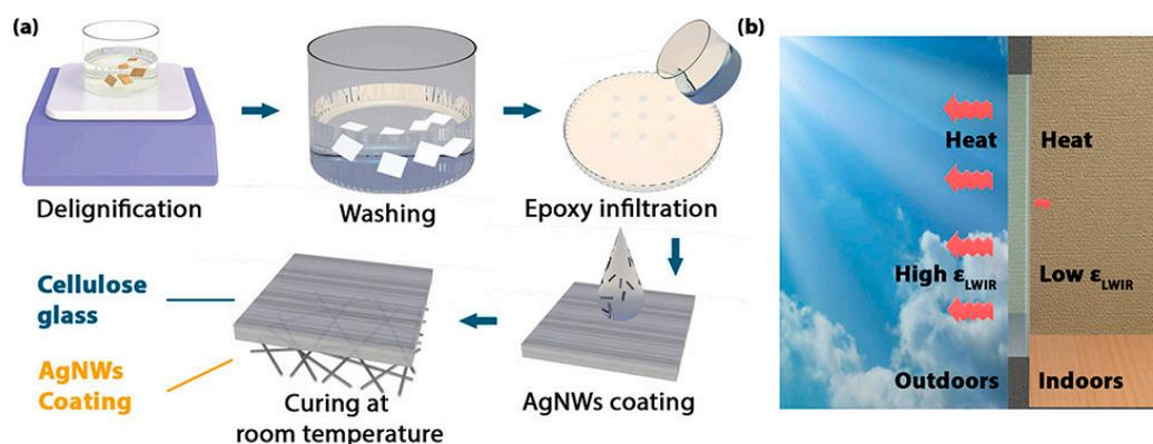
**Figure 27.** (a) Schematic manufacturing procedures of the radiative cooling transparent bamboo; (b) schematic demonstration of the working mechanism of the radiative cooling transparent bamboo. AgNWs = silver nanowires;  $\epsilon_{LWIR}$  = long-wavelength infrared emissivity. Reprinted with permission from [43], copyright 2021, American Chemical Society.
