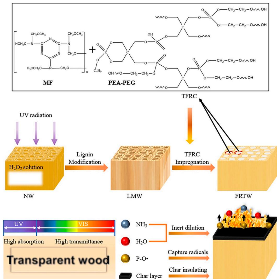
**Figure 34.** Schematic illustration of the preparation of flame-retardant transparent wood (FRTW), together with the demonstration of its optical and flame-retardant properties. NW = natural (pristine) wood; LMW = lignin-modified wood; MF = melamine–formaldehyde resin; PEA-PEG = flame-retardant product obtained by reacting poly(ethylene glycol) with cyclic phosphate ester; TFRC = transparent flame-retardant resin system. Reprinted with permission from [49], copyright 2022, John Wiley & Sons.
