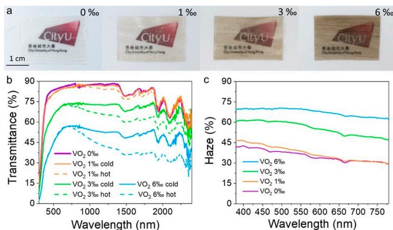
**Figure 17.** (a) Thermochromic transparent wood film (TTWF) with different concentrations of W-doped VO<sub>2</sub> (0, 1, 3, and 6‰ from left to right); (b) temperature-dependent optical transmittance spectra of VO<sub>2</sub>-TTWF; and (c) optical transmittance haze of VO<sub>2</sub>-TTWF. VO<sub>2</sub> X‰ cold and hot refer to transmittance measured after thermal switching from cold to hot state. Reprinted with permission from [39], copyright 2021, American Chemical Society.
