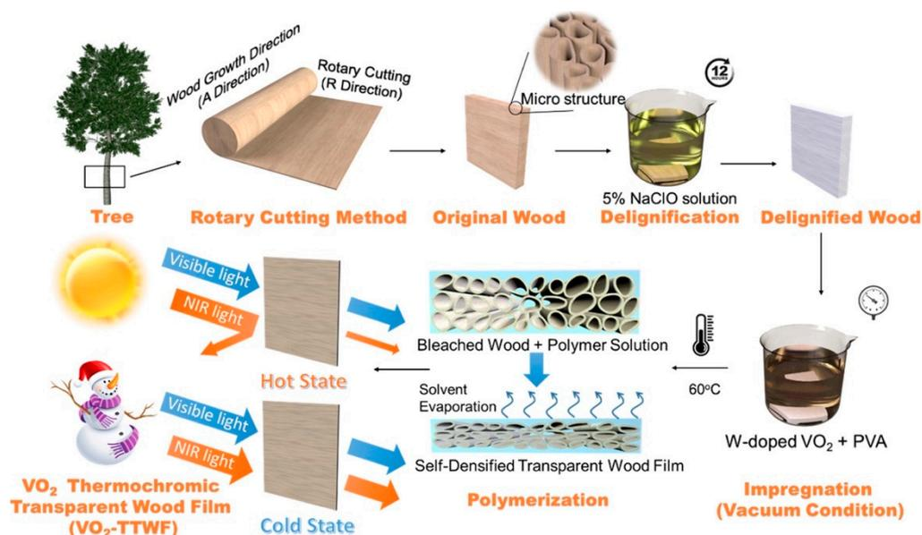
**Figure 16.** Scheme of the process for obtaining thermochromic transparent wood films containing VO<sub>2</sub> nanoparticles (VO<sub>2</sub>-TTWF). Reprinted with permission from [39], copyright 2021, American Chemical Society.
