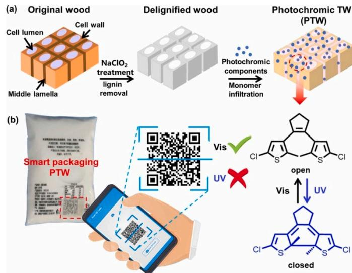
**Figure 14.** Schematic illustration of the preparation and application of smart photochromic transparent wood (PTW). (a) The fabrication process of the PTW. (b) Potential smart packaging applications of PTW. Reprinted with permission from [38], copyright 2022, Elsevier.
