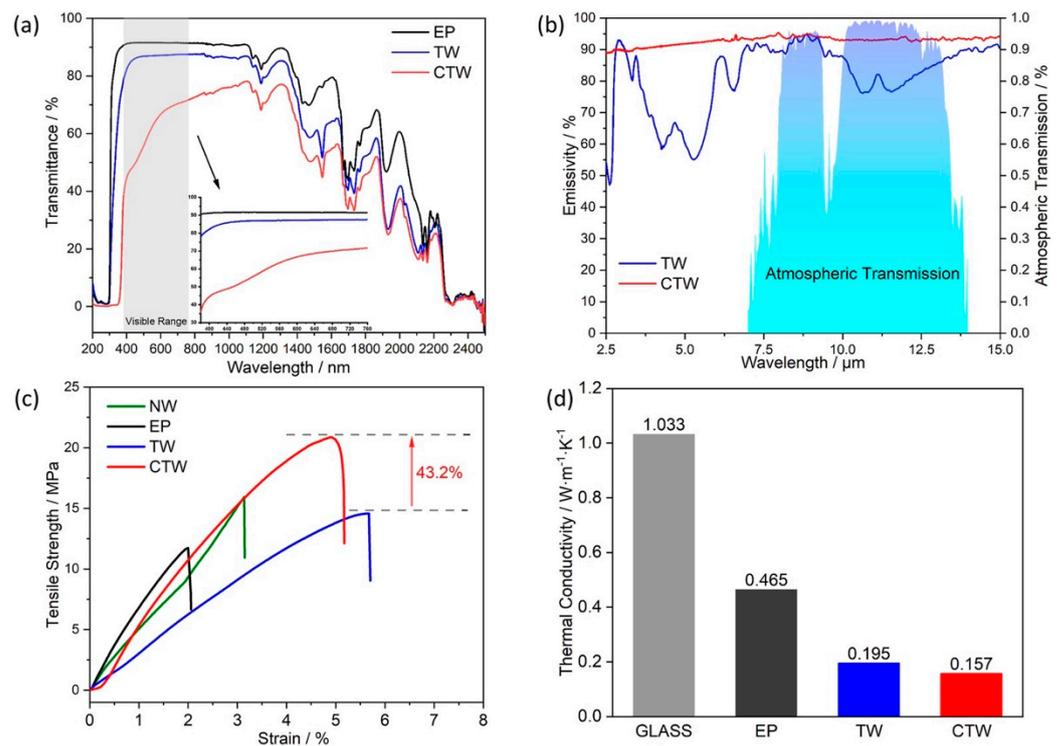
**Figure 25.** (a) Transmittance vs. wavelength curves of cured epoxy resin (EP), uncoated transparent wood (TW), and ZnO-coated transparent wood (CTW); (b) emissivity spectrum of TW and CTW within the long-wavelength infrared region; (c) stress–strain curves of natural wood (NW), EP, TW, and CTW; (d) thermal conductivity of glass, EP, TW, and CTW. Reprinted with permission from [42], copyright 2022, Elsevier.
