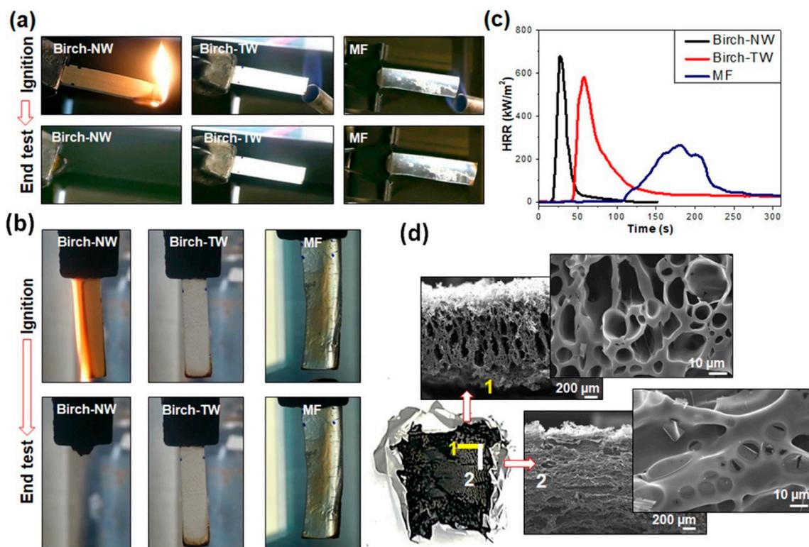
**Figure 38.** Flame spread test snapshots (a) in horizontal, (b) in vertical configuration, and (c) heat release rate vs. time curves for pristine birch wood (Birch-NW), flame-retardant birch wood (Birch-TW), and cured melamine–formaldehyde resin (MF); (d) cross-section SEM micrographs of the residues of Birch-TW in two perpendicularly oriented planes. Reprinted from [50] under CC-BY license.
