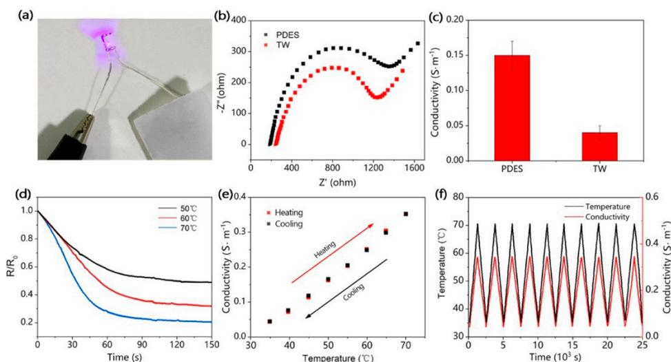
**Figure 23.** Electrical properties and temperature sensing performance of transparent wood (TW). (a) Digital image to demonstrate that the TW can illuminate an LED bulb. (b) Electrochemical impedance spectroscopy (EIS) plots of the deep eutectic solvent polymer (PDES) and TW. (c) Plots of
