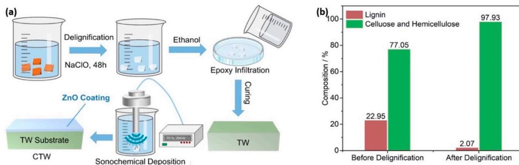
**Figure 24.** (a) Schematic manufacturing procedures of coated transparent wood (CTW); (b) chemical compositions of balsa wood before and after delignification. Reprinted with permission from [42], copyright 2022, Elsevier.
