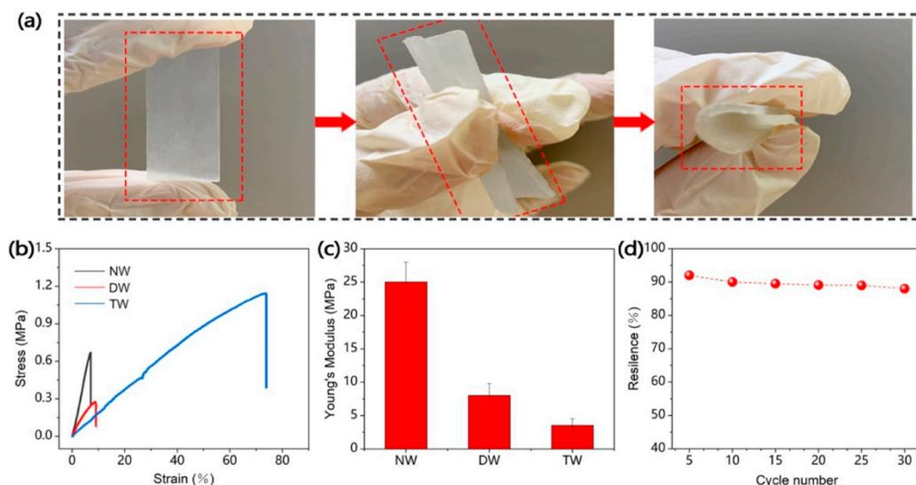
**Figure 21.** Mechanical properties of transparent wood. (a) Transparent wood becomes highly flexible upon bending. (b) Typical stress–strain curves of natural (pristine) wood (NW), delignified wood (DW), and transparent wood (TW). (c) Young's modulus of NW, DW, and TW. (d) Resilience of the TW at different cycle numbers measured under 40% strain. Reprinted permission from [41], under CC-BY license.
