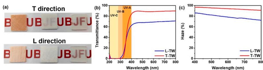
**Figure 32.** Optical properties of the transparent wood (TW). (a) From left to right, transverse (T direction) and longitudinal (L direction) digital images of wood, delignified wood, and transparent wood (thickness = 2 mm). (b,c) Total transmittance and haze of transverse (T-TW) and longitudinal (L-TW) transparent wood (thickness = 2 mm). Reprinted with permission from [47], copyright 2022, Elsevier.
