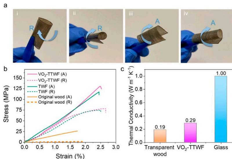
**Figure 18.** (a) VO<sub>2</sub>-TTWF was folded and rolled in both A (axial) and R (radial) directions, as shown in the images i-iv. (b) Stress–strain curves of VO<sub>2</sub>-TTWF, TWF, and original wood in A and R directions. (c) Comparison of thermal conductivity of VO<sub>2</sub>-TTWF, transparent wood, and glass. Reprinted with permission from [39], copyright 2021, American Chemical Society.
