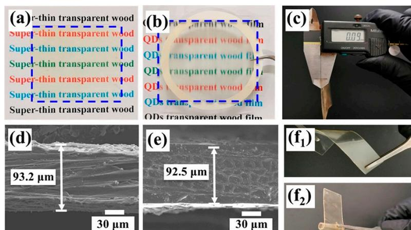
**Figure 12.** (a,b) Superthin transparent wood films placed directly on substrate and 10 mm above the substrate, respectively. (c) Thickness of the superthin transparent wood films measured with vernier calipers. (d,e) Thickness of superthin transparent wood films confirmed by SEM. (f<sub>1</sub>,f<sub>2</sub>) The flexibility of a transparent wood film, rolled in different directions. Reprinted with permission from [37], copyright 2022, American Chemical Society.
