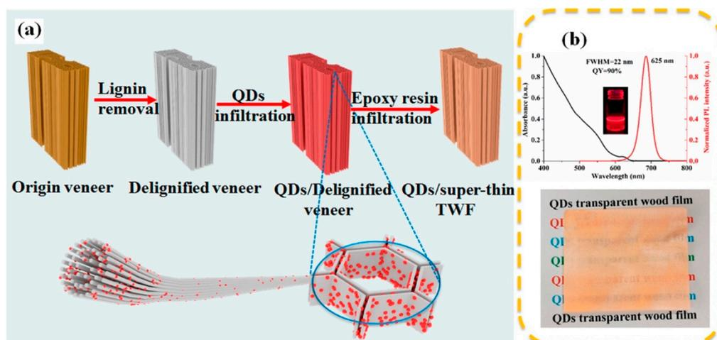
**Figure 11.** (a) Schematic illustration of preparation of QD/superthin transparent wood films (TWFs). (b) Luminescence and absorption spectra of the red QD solution (top) and a digital image of the QDs/delignified veneer (bottom). Reprinted with permission from [37], copyright 2022, American Chemical Society.
