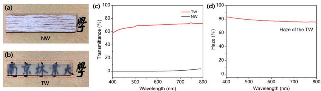
**Figure 22.** Comparison of optical properties between natural (pristine) wood (NW) and transparent wood (TW). (a,b) Digital images of the NW and TW laid on the same pattern. (c) Optical transmittance of the NW and TW. (d) Optical haze of the TW. Reprinted permission from [41], under CC-BY license.
