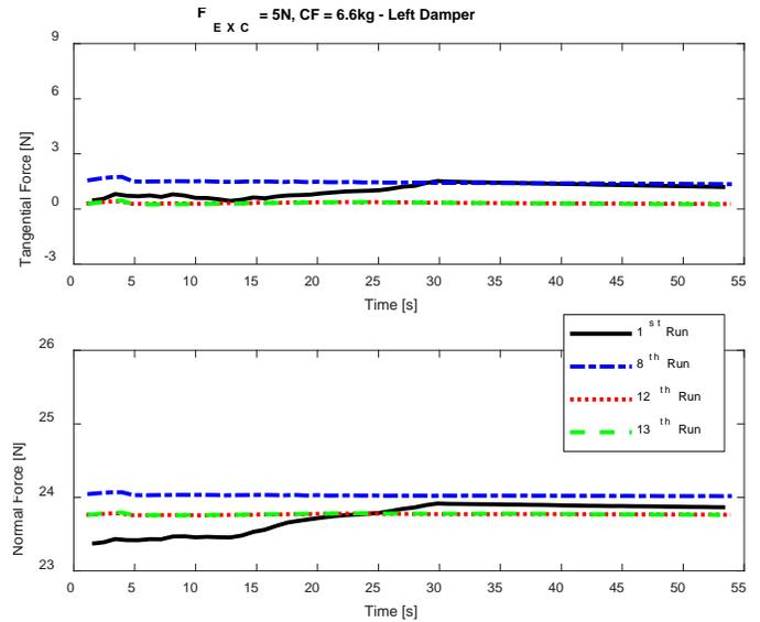
**FIGURE 17:** THE EVOLUTION OF STATIC CONTACT FORCES ON THE LEFT DAMPER IN DIFFERENT RUNS FOR THE 4<sup>TH</sup> SUBSET ( $F_{EXC} = 5 \text{ N}$ ,  $CF = 6.6 \text{ kg}$ )
