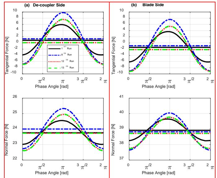
FIGURE 9: CONTACT FORCES ON THE LEFT DAMPER FOR THE 4<sup>TH</sup> SUBSET ( $F_{\text{EXC}} = 5 \text{ N}$ ,  $\text{CF} = 6.6 \text{ kg}$ )
