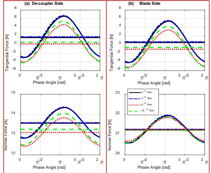
**FIGURE 14:** CONTACT FORCES ON THE LEFT DAMPER FOR THE 6<sup>TH</sup> SUBSET ( $F_{EXC} = 5\text{ N}$ ,  $CF = 3.6\text{ kg}$ )
