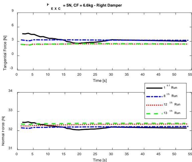
**FIGURE 16:** THE EVOLUTION OF STATIC CONTACT FORCES ON THE RIGHT DAMPER IN DIFFERENT RUNS FOR THE 4<sup>TH</sup> SUBSET ( $F_{EXC} = 5 \text{ N}$ ,  $CF = 6.6 \text{ kg}$ )
