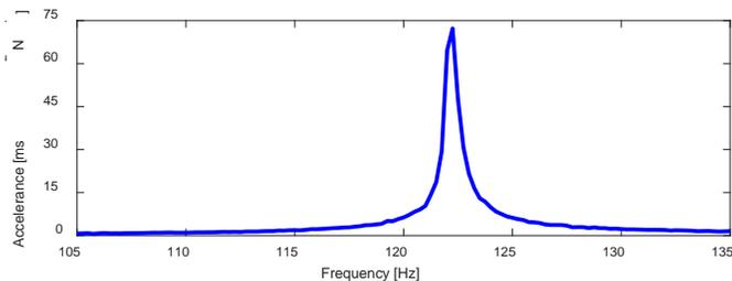
**FIGURE 4:** LINEAR RESPONSE OF THE BLADE WITHOUT DAMPERS
