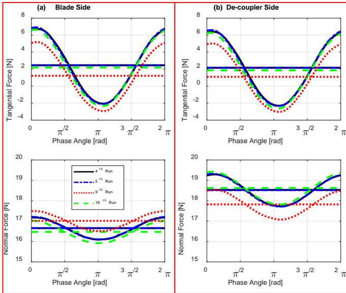
**FIGURE 13:** CONTACT FORCES ON THE RIGHT DAMPER FOR THE 6<sup>TH</sup> SUBSET ( $F_{EXC} = 5\text{ N}$ ,  $CF = 3.6\text{ kg}$ )
