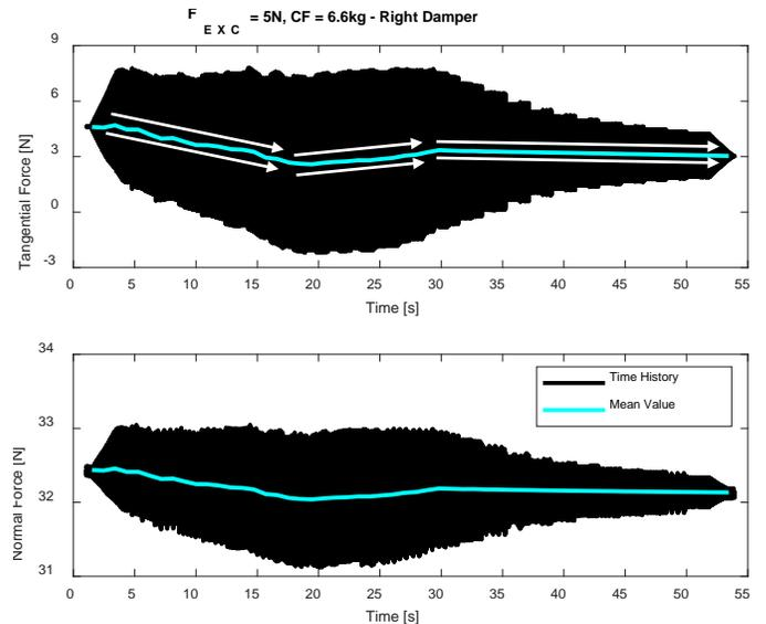
**FIGURE 15:** THE EVOLUTION OF THE CONTACT FORCES ON THE RIGHT DAMPER IN THE 1<sup>ST</sup> RUN OF THE 4<sup>TH</sup> SUBSET ( $F_{EXC} = 5\text{ N}$ ,  $CF = 6.6\text{ kg}$ )
