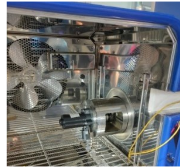
Fig.7 The slender PM motor inside the climatic chamber.
