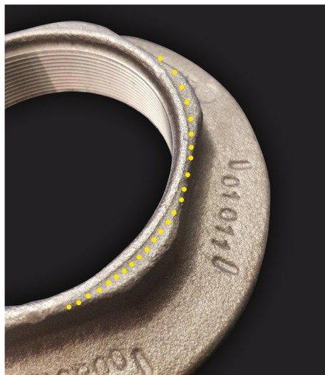
Fig. 5 Effects of elastic subsidence of the die on the forged part
