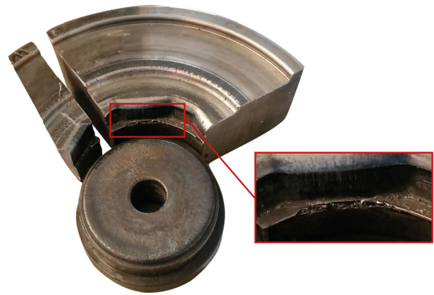
Fig. 2 The damaged section of the die
