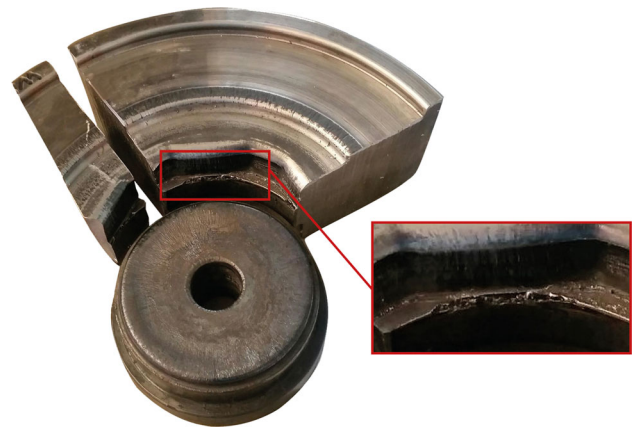
Fig. 2 The damaged section of the die
