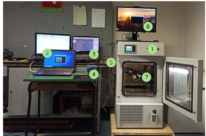
Fig. 5. Setting of the laboratory tests. (1) marks the climatic chamber, whose behavior was monitored via two screens (2). A laptop with the 3-D Viewer in execution is highlighted with (3), while (4) displays the interrogator. The Raspberry Pi 1 is highlighted by (5), and its operations can be monitored by screen (6). Finally, (7) indicates the monitored test sample with the FBG sensor.
