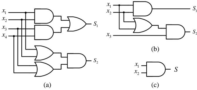
Fig. 4: Approximate compressors with constant compensation. (a) AC\_42, (b) AC\_32, (c) AC\_21.
