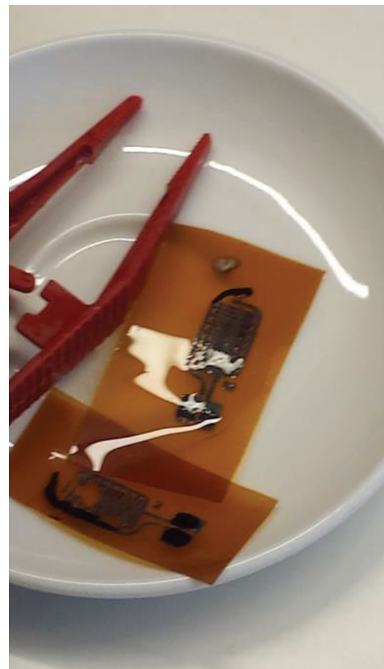
Figure 10. Circuits etched on copper laminated films (Photo: Alvis Mattozzi)
