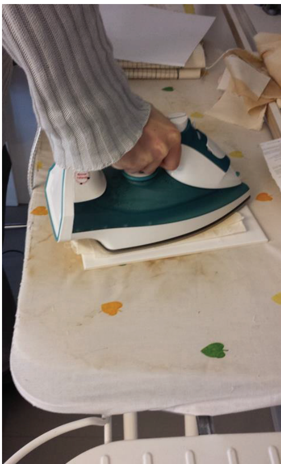
Figure 12. The transfer of laser-printer ink from glossy paper to copper laminated film. A ceramic tile can be spotted below the cloth protecting the glossy-paper-printed-circuit-film coupling (Photo: Alvis Mattozzi)
