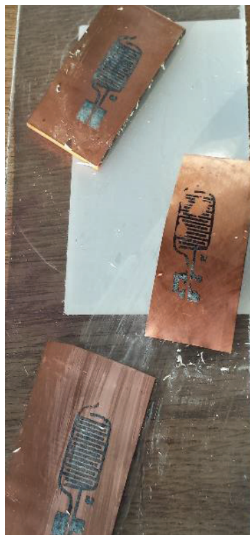
Figure 7. The subtractive method of etching a printed circuit board (our drawings)
