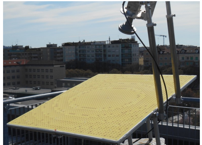
Fig. 4. Manufactured prototype mounted in the outdoor test range.
