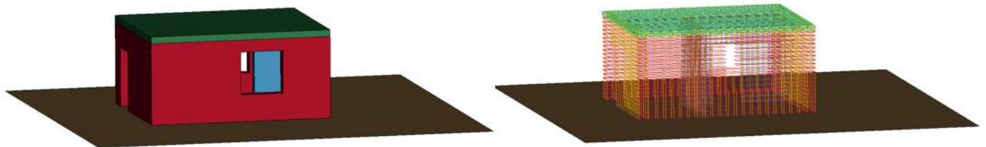
Figure 3. Details of the complete 3D model made with LS-DYNA and details of the steel armor.
