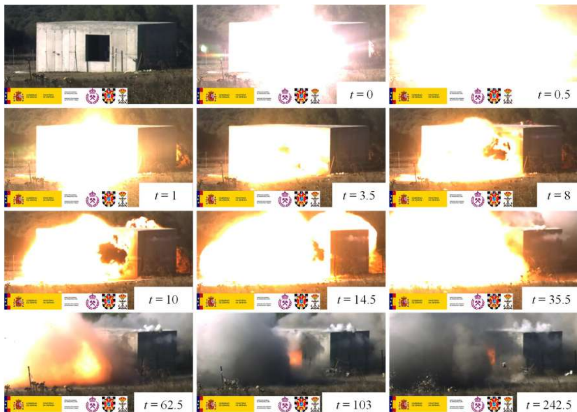
Figure 7. Sequence of images obtained with HSC in trial T7: PG2. Time in milliseconds; the reference time is the first frame of the video where the detonation is observed.
