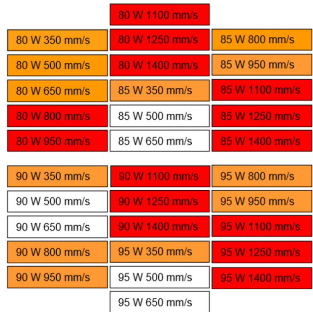
Fig. 3. SST parameters explored for the first screening. The SSTs with strong discontinuities are reported in red and SSTs with low quality are marked in orange. (For interpretation of the references to colour in this figure legend, the reader is referred to the web version of this article.)
