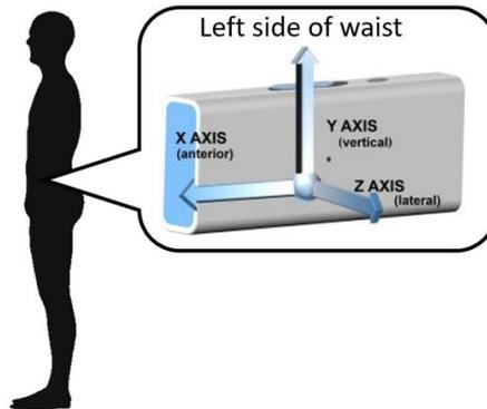
Figure 1: Sensor position and axes orientation in the REMPARK dataset. The front, vertical, and lateral (left) direction corresponds to the x-axis, y-axis, and z-axis of the sensor reference system, respectively.
