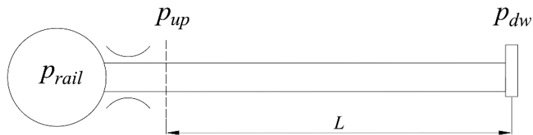
Figure 5. Scheme of the hydraulic model.
