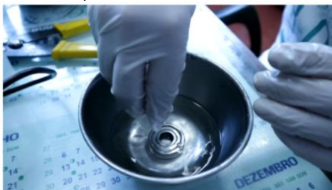
Fig. 5. Grease removal process from the bearings.
