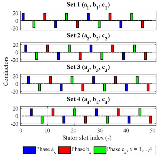
Fig. 2. Conductors' distribution of the 12-phase IM.
