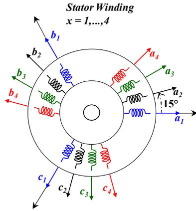
Fig. 1. A view of the magnetic axes of the asymmetrical 12-phase IM.
