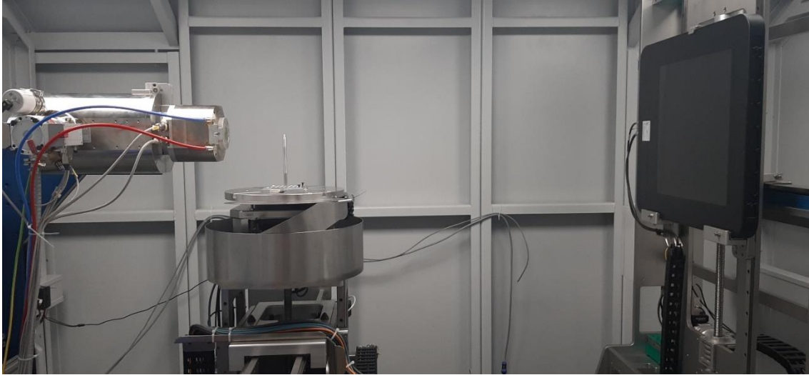
13 14 15 16 17 18 19 20 21 22 23 24 25 26 27 28 29 30 31 32 Figure 2: Details of the micro-CT equipment showing its main components: the X-ray tube, the stage that holds the 33 specimen, and the flat detector panel. 34 35 36
