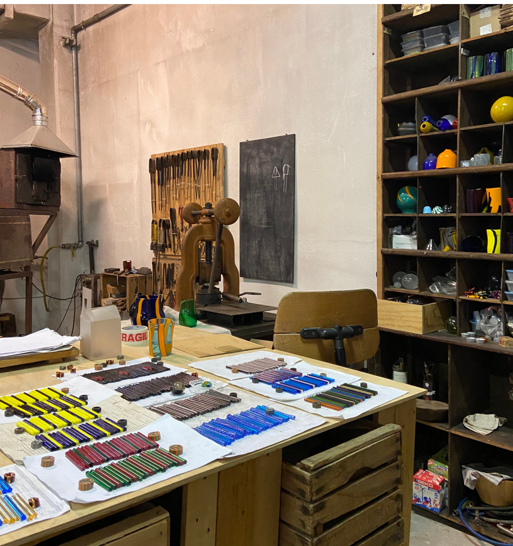
Figure 2. Joga Glass workshop. On the table, combinations of glass rods prepared to be heated and picked-up with the roll-up technique. The different arrangements of colours allow to obtain different chromatic effects. The combinations are almost infinite and the result is always different.
