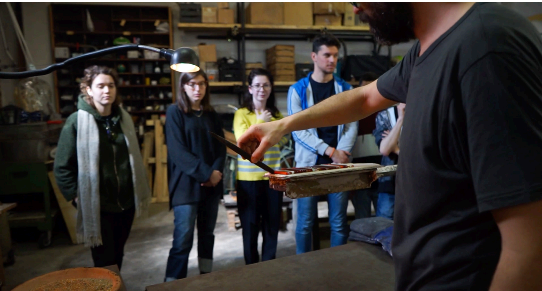
Figure 4. The glass master giving a demonstration to the workshop's participants of the first step for the creation of a vase. The combined rods are placed on a ceramic plate to be rolled-up and then blown to get the final shape.
