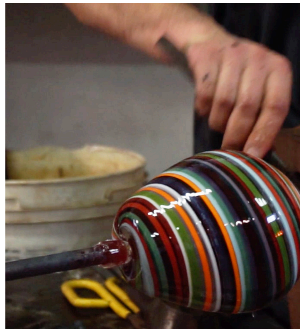
Figure 7. Final modelling of the glass object. As in previous steps the glass master is using his manual ability and experience to define the shape. The starting rods are clearly visible but they have been twisted to create a unique pattern.
