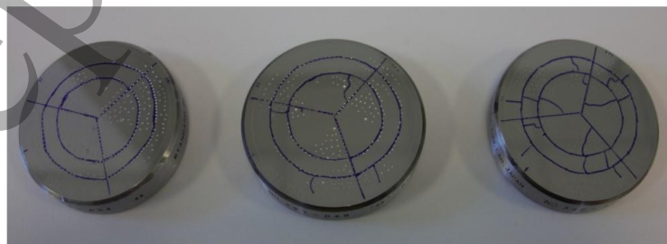
Figure 3: The three hardness blocks used in the measurements.
