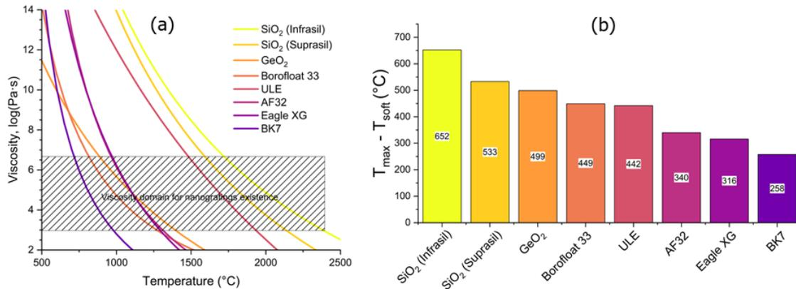
Fig. 2. (a) Viscosity as a function of temperature for a variety of commercial and typical glasses, along with an estimated domain of nanogratings existence from  $T_{soft}$  ( $\eta = 10^{6.6}$  Pa·s) to  $T_{max}$  ( $\eta = 10^{3.0}$  Pa·s). (b) Temperature difference ( $T_{max} - T_{soft}$ ) as a function of glass composition. A larger value suggests a wider processing window (with respect to temperature) to form nanogratings.
