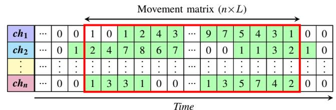
Fig. 2. Example of *movement* segmentation performed on  $n$  acquisition channels. Row sequences marked in green represent channels activations, while the red box segments the multi-channel sequence which satisfies the  $GFT$  condition ( $GFT = 2/n$ ).
