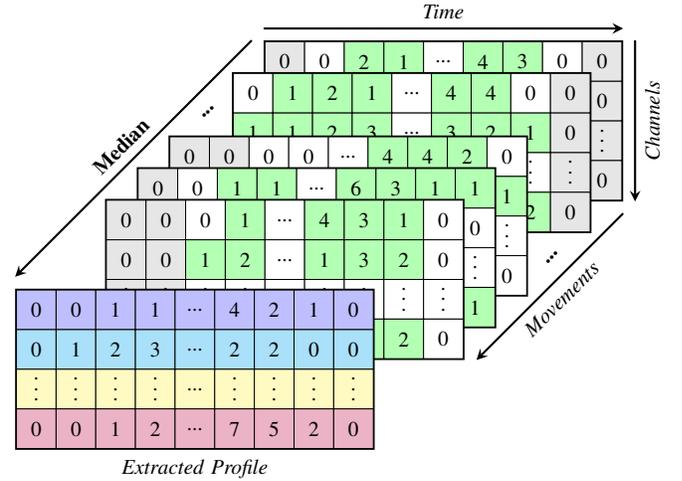
Fig. 4. Example of *movements* alignment: *movement* matrices are aligned, maximizing the mutual cross-correlation. Columns marked in gray are added to equalize matrices dimension. Sequences highlighted in green represents channels' activity.
