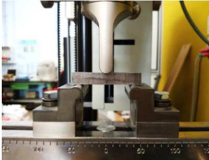
Fig. 19. Transversal break test device (TRS)
