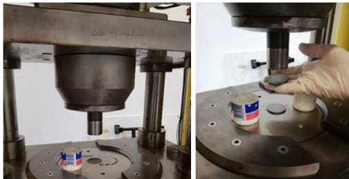
Fig. 6. Powder deposition in the mold and cylindrical sample
