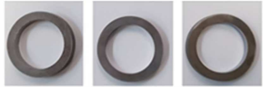
Fig. 9. Toroidal specimens after milling
