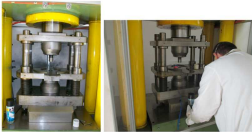
Fig. 5. 200 tons press adopted to realize the specimens
