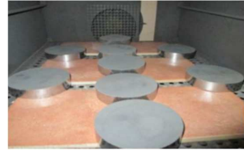
Fig. 7. Specimens of heat treatment in the oven
