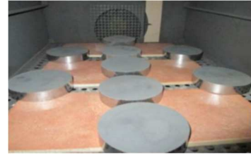
Fig. 7. Specimens of heat treatment in the oven
