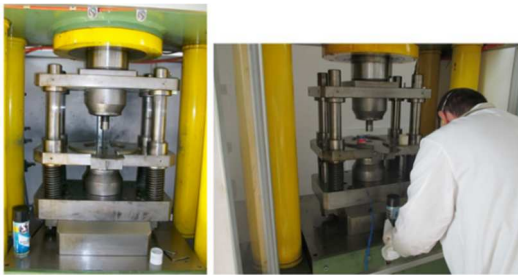
Fig. 5. 200 tons press adopted to realize the specimens
