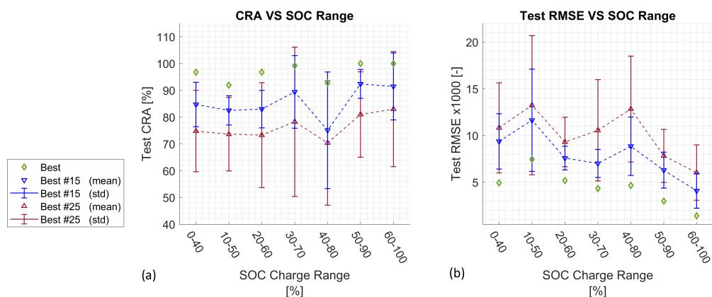
**Figure 11.** Sensitivity analysis of the best 15 and 25 neural networks according to the RMSE on the testing dataset for  $L_{opt} = 40\%$ . (a) CRA trend depending on the input SOC window selected. (b) Test RMSE  $\times 1000$  depending on the input SOC window selected.
