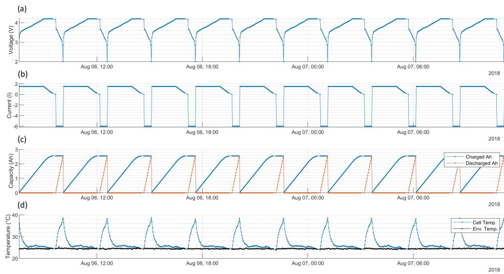
**Figure 2.** Example of constant current constant voltage charge profiles measured by Sandia National Laboratories during the performed experimental cell aging campaign. The cell operating parameters measured during the tests are (a) cell voltage (V), (b) current (A), (c) charged and discharged capacity (Ah), and (d) cell and environmental temperature (°C).
