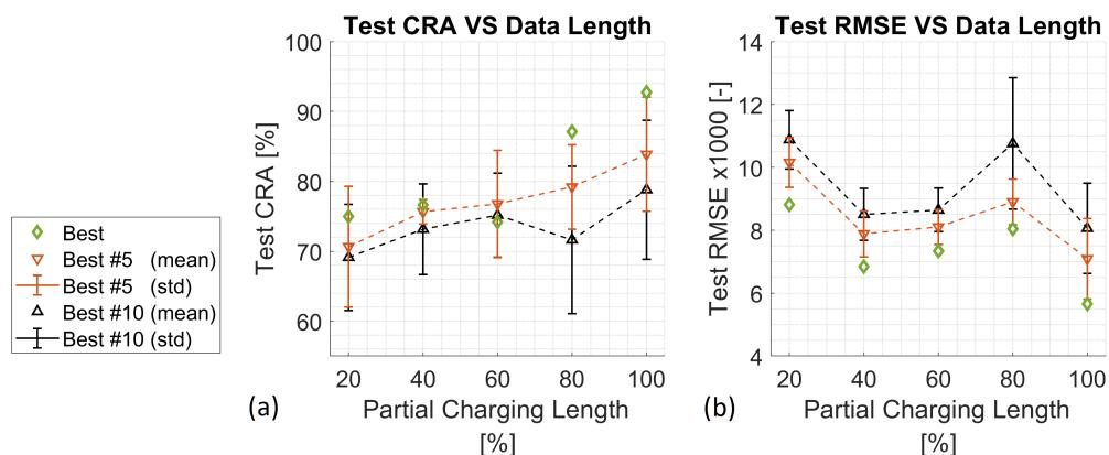
**Figure 8.** (a) CRA sensitivity analysis of the best one, five and 10 trained networks according to the RMSE on testing dataset. (b) RMSE sensitivity analysis of the best one, five and 10 trained neural networks according to the RMSE on testing dataset. For partial charging lengths, the minimum RMSE is equal to 0.0068 corresponding to 40% data length.
