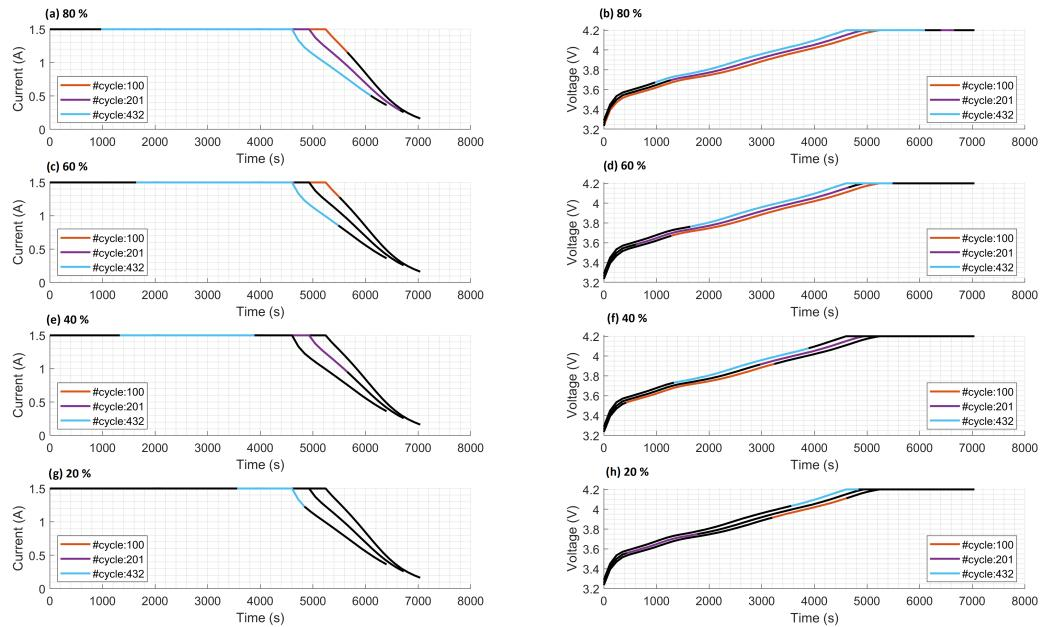
**Figure 5.** Operating current and voltage of few partial charging segments. (a,b) are operating current and voltage of the partial charging length equal to 80%. (c,d) are operating current and voltage of the partial charging length equal to 60%. (e,f) are operating current and voltage of the partial charging length equal to 40%. (g,h) are operating current and voltage of the partial charging length equal to 20%. In the graphs, the black lines is the full size of data (equal to 100% of length).
