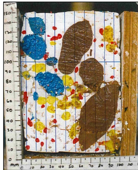
Figure 1. Scanlines (blue) traced on 42% physical bimrock model (original of monochrome image of Figure 3 of Medley's [43] work).
