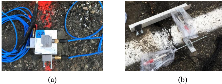
Figure 24: Mono-axial accelerometers (a); LVDT at joint (b)
