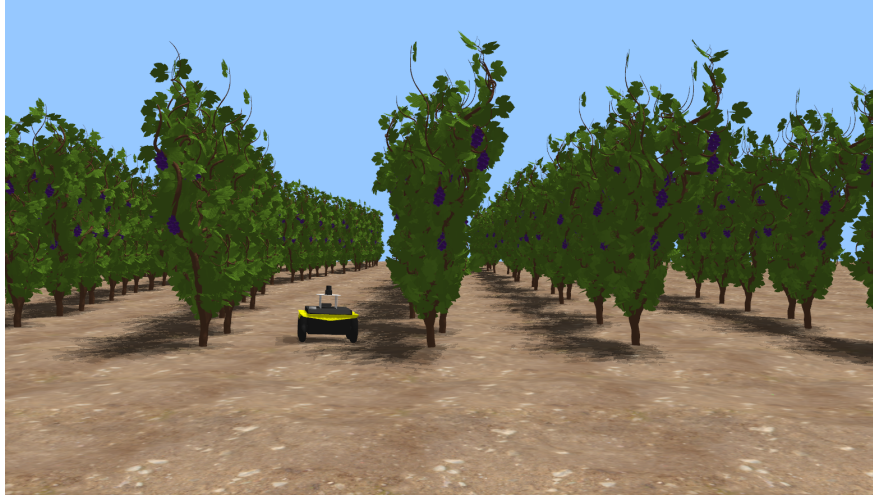
Figure 2: The robot is placed in a vineyard environment with realistic terrain profile. In testing rows, curves and plant gaps are introduced to validate the agent in conditions comparable to real-world challenging scenarios.
