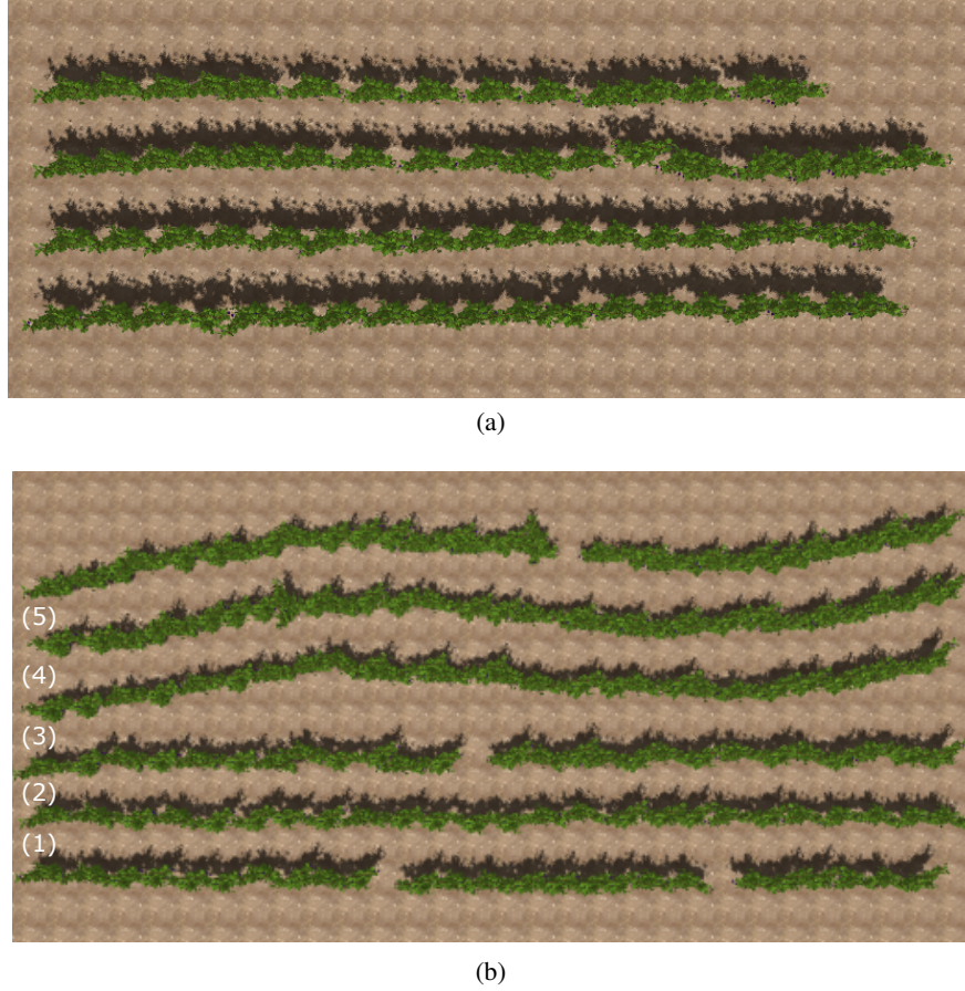
Figure 5: Training (a) and testing (b) simulation environments. Intentional gaps and curves are introduced in (b) to provide a challenging environment for the agent. Testing rows are numbered as referenced in the results section.
