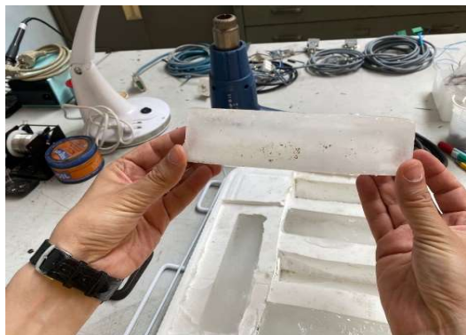
Figure 5– Resin mold and the plain ice specimen
