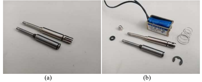
Fig. 19 - The original and FeSi2.9 plunger (a) and solenoid closing system (b)
