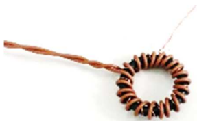
Fig. 5 - FeSi2.9 Toroid: size and shape not fully compliant with the IEC 60404 series standards
