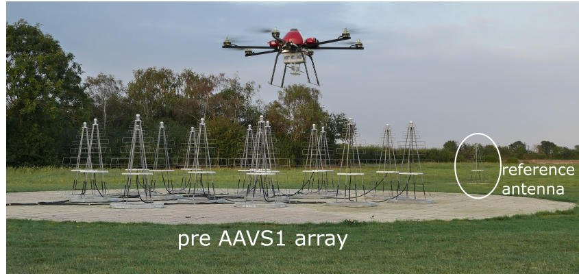
Fig. 4.1 The UAV flies over the array under test i.e., the Pre - Aperture Array Verification System. On the right (white circle): reference antenna used for phase reconstruction. Picture from [34].
