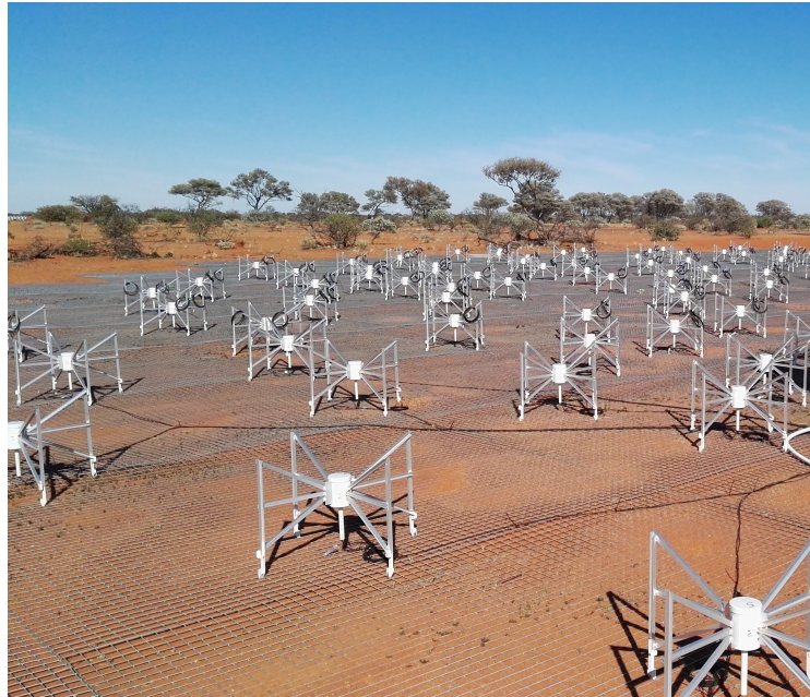
Fig. 3.4 Bow-tie dipoles of the Engineering Development Array 2 (EDA2).
