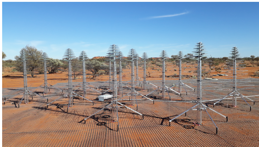
Fig. 3.3 Log-periodic elements of the Aperture Array Verification System 1.5 (AAVS1.5).
