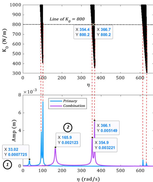
Fig. 7 JBA results for  $K_0 = 800$  (N/m)
