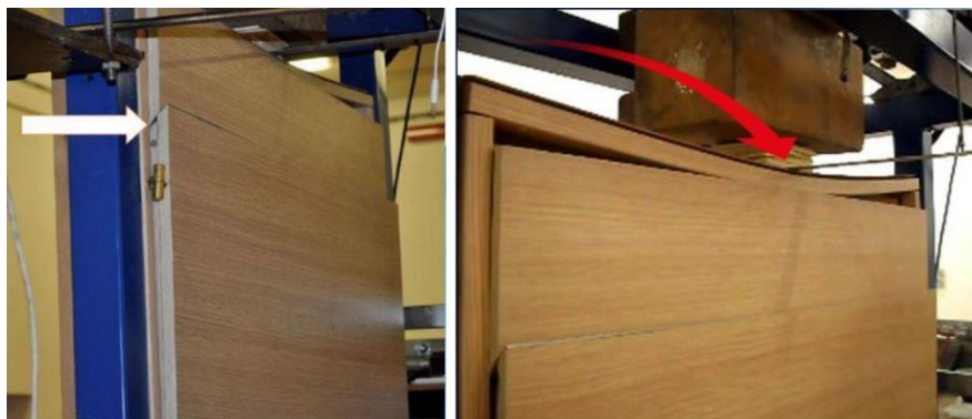
Fig. 49: Emergency System for door opening in critical condition proposed by LF System Italia s.r.l.s. [150].
