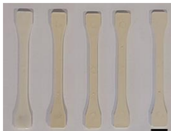
Figure 2. Injection-molded specimens at different ZTC content: from left to right the ZTC wt% varies from 0 to 40% (the dimensional marker is equal to 1 cm).
