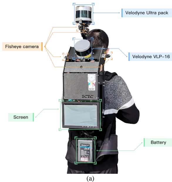
Figure 2. Illustration of indoor LiDAR-based indoor point cloud. (a) multi-beam laser scanning sensor model. (b) the high-accuracy reference TLS point cloud.
