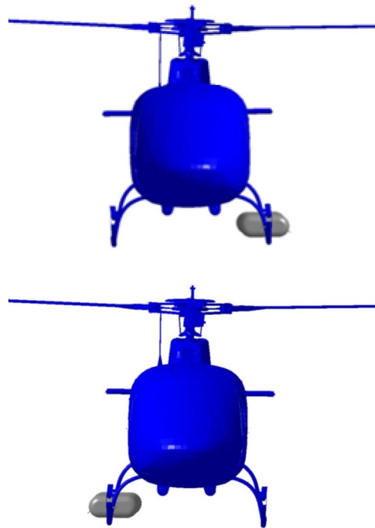
Fig. 1 Asymmetrical single-basket configurations
