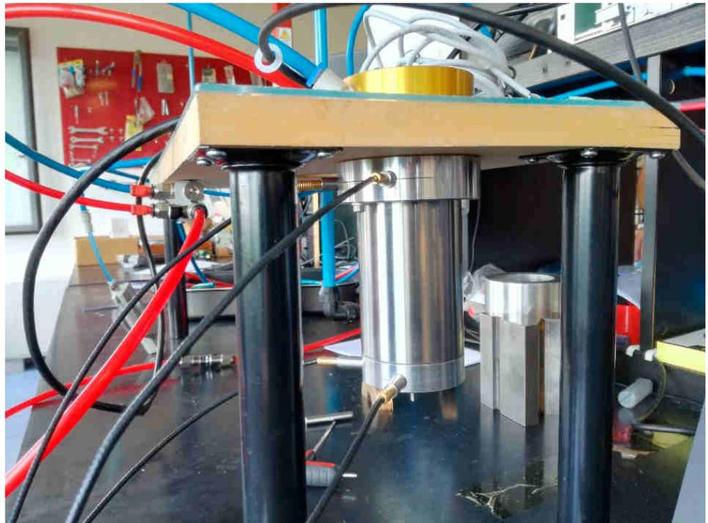
**Figure 1.** The electro-spindle under test.
