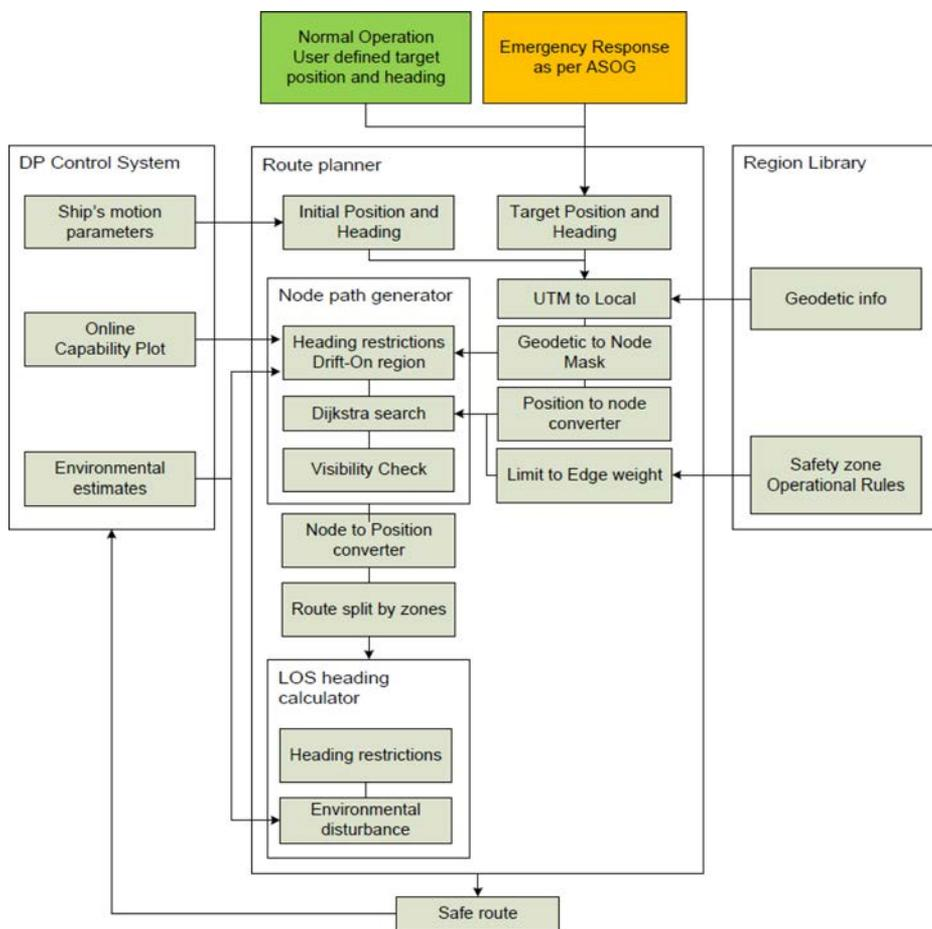
Fig. 31. Overview of the safe maneuver planning algorithm.
