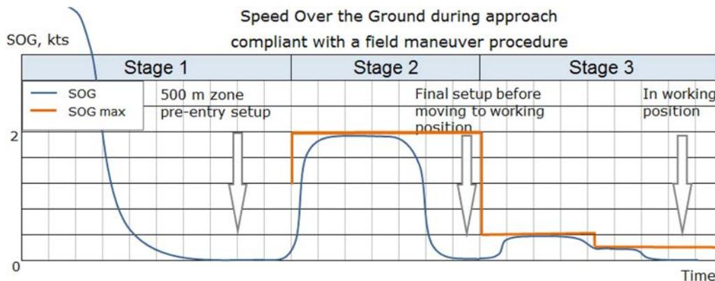
Fig. 2. SOG along the approach trajectory as intended by a set of field safety instructions.
