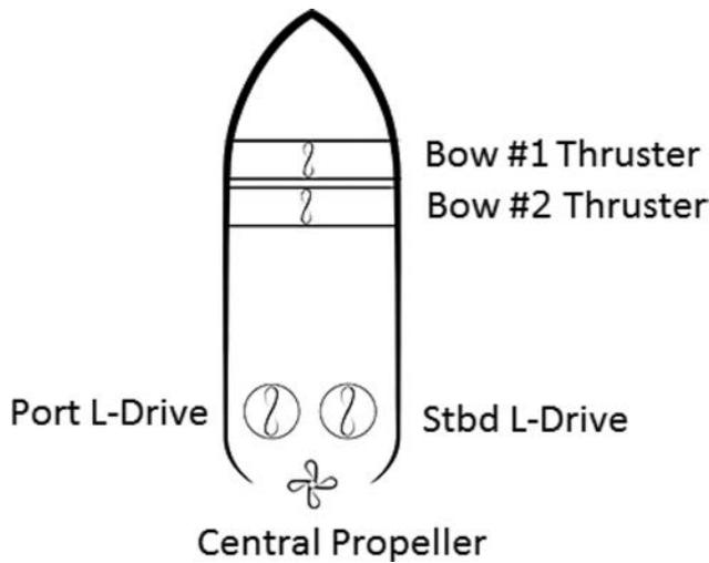
Fig. 9. Thruster configuration of Platform Supply Vessel *BOURBON Liberty 150* series.
