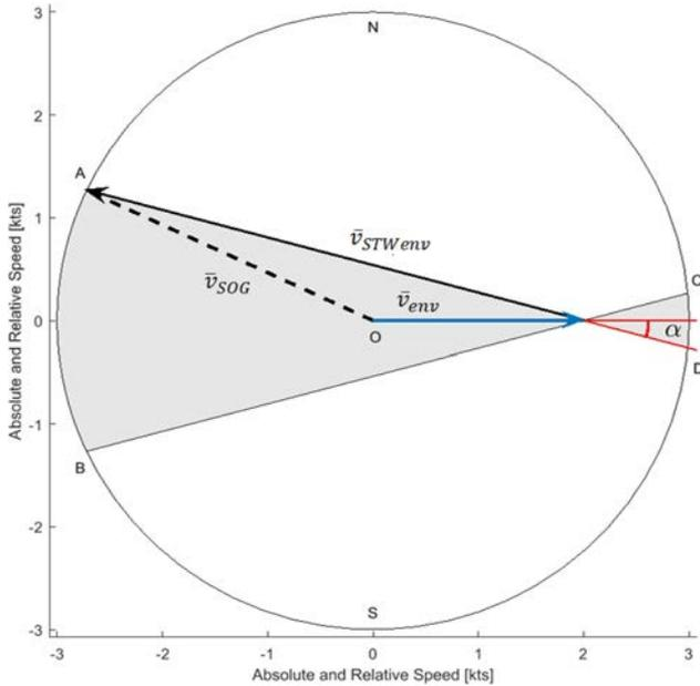
Fig. 26. Polygon in gray denotes the boundaries of allowable SOG with the heading restrictions applied. The  $\varphi_{env}$  is  $90^\circ$ . Maximum SOG is set to 3 kn in this example.  $v_{env}$  is the equivalent speed vector derived from  $F_{env}$ . All vectors are applied at the ship's center of mass.
