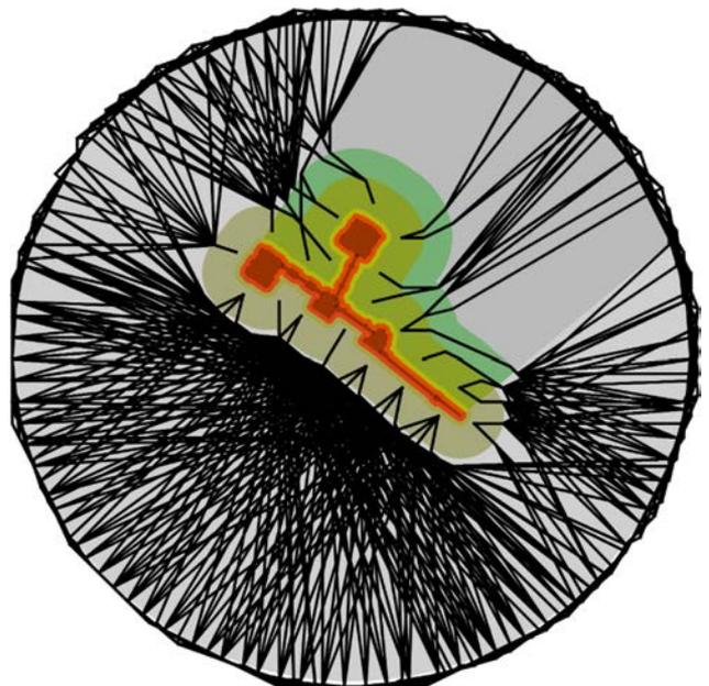
Fig. 29. Result of plotting 2000 approach trajectories with a connectivity method described in Section IV-C for the UD region, 16 neighbor node reach,  $\varphi_{env} = 225^\circ$ .
